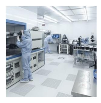
In particular, the work was carried out at **FBK's MicroNano Facility**'s "Clean Room", a laboratory with cleaning procedures similar to those of an operating room.
