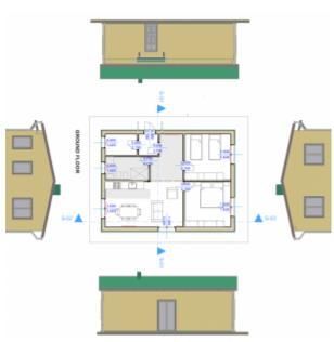
IsoIMAX is expected to build an 80 sqm laboratory-building in Barnaul, south-western Siberia, designed according to the steeIMAX® construction model, a system patented by Cogi that enables "dry" construction in residential buildings, with metal supporting frames, which cut down construction time, costs and complexity compared to traditional building systems.
